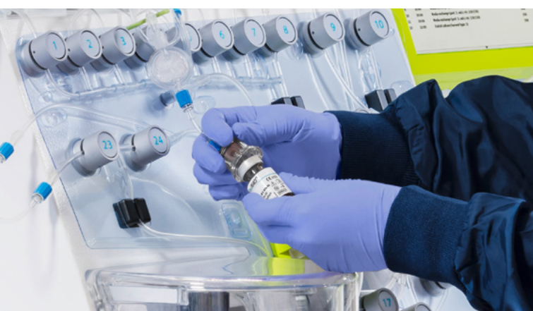
Figure 1: Connecting CliniMACS CD34 Reagents to the CliniMACS Prodigy.
